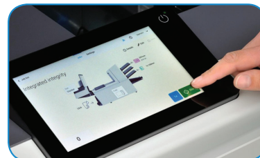
Color 7" touchscreen control panel with graphical interface and paper/envelope presence sensors
